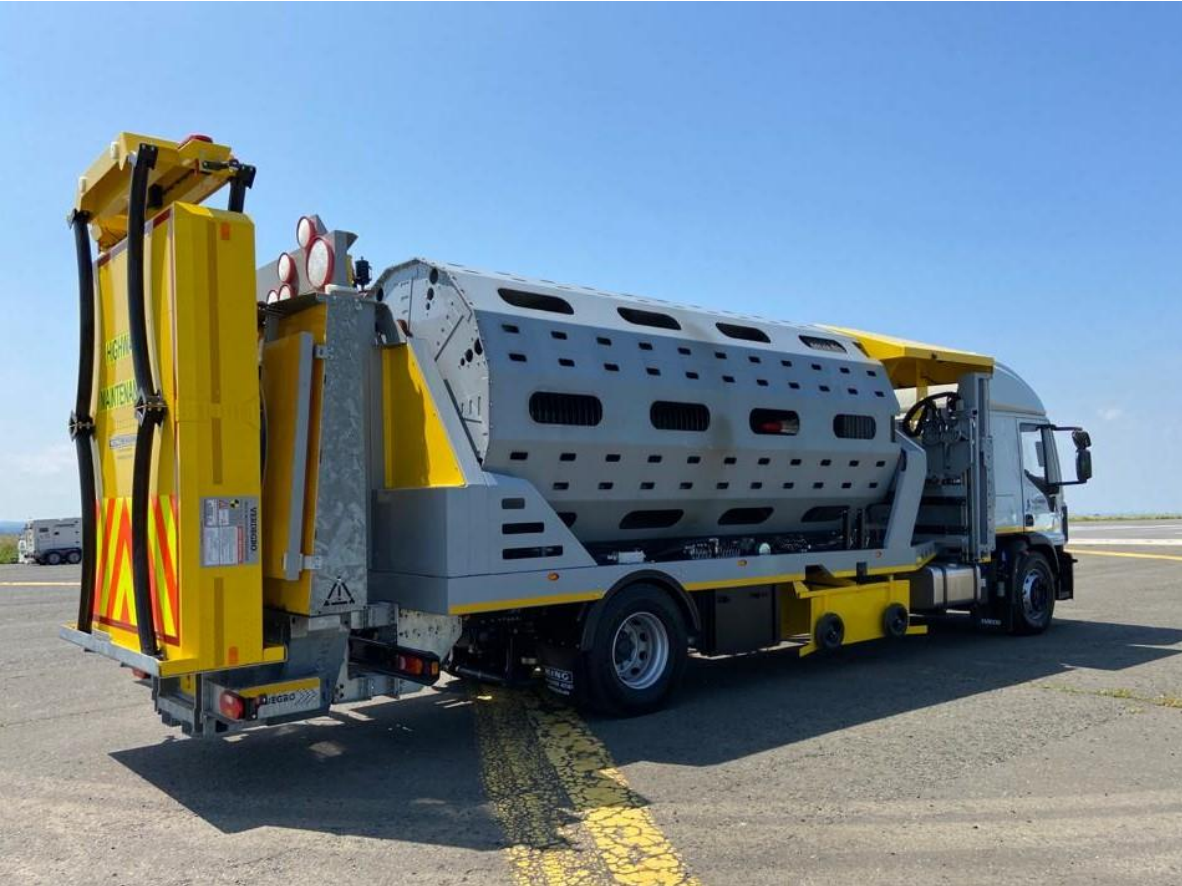
Figure 24 – National Highways’ second automated cone-laying vehicle xlvi
