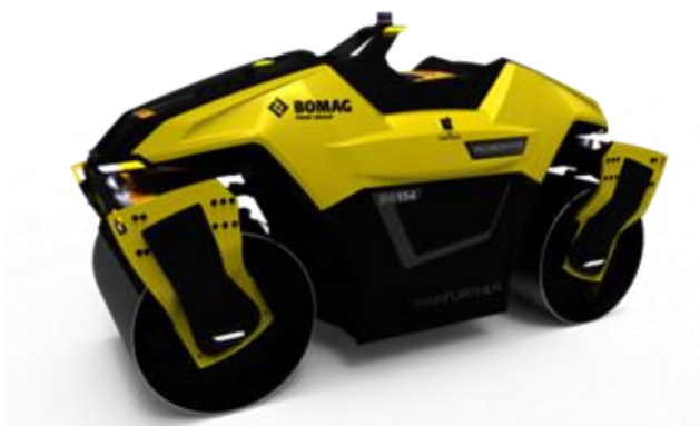
Figure 4 - BOMAG Robomag Autonomous Roller
