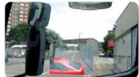
FRESNEL Lens showing a family saloon car in the lorry's blind spot.
